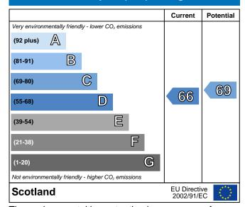
The environmental impact rating is a measure of a home's impact on the environment in terms of carbon dioxide (CO<sub>2</sub>) emissions. The higher the rating the less impact it has on the environment.
