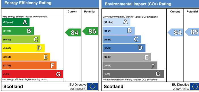
The energy efficiency rating is a measure of the overall efficiency of a home. The higher the rating the more energy efficient the home is and the lower the fuel bills are likely to be. The environmental impact rating is a measure of a home's impact on the environment in terms of carbon dioxide (CO<sub>2</sub>) emissions. The higher the rating the less impact it has on the environment.
