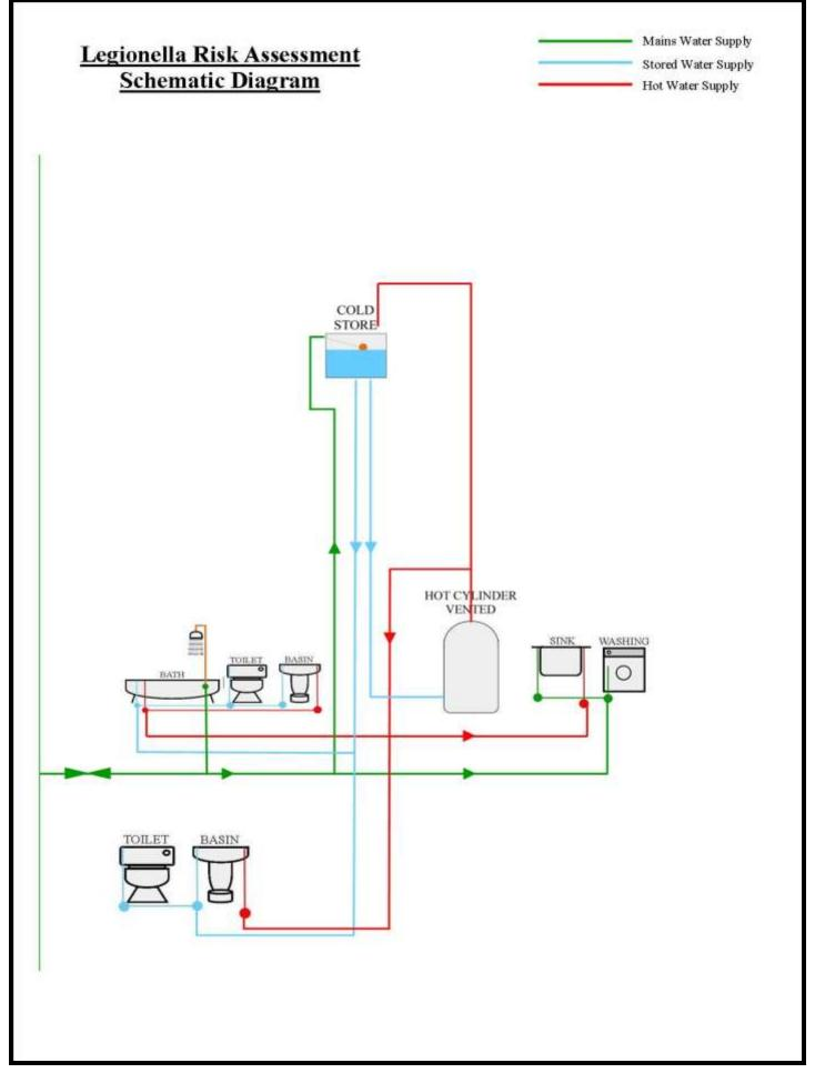
This schematic is a simplified illustration of the layout of the water system based on what fixtures and pipework were visible at the time of the inspection, it provides only an indication of scale. Whilst every effort has been made to ensure the schematic diagrams are as accurate as possible Contract Heating Ltd. cannot gaurantee their accuracy.
